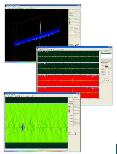
TecView™ EC has all the required features to make TecScan's Bearing Inspection System a truly time saving and easy to use solution for your bearing inspection needs. With features that permit the user to set multiple alarms, display the inspection in track mode, and generate print reports, TecView™ EC is truly tailored to bearing inspections. In addition most commercial eddy current units can be integrated to the system thus enabling it to meet clients' requirements.
