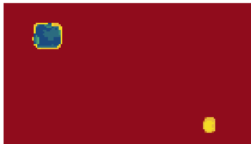
Fig. 9. Time-of-flight C-Scan calculated from the 10 MHz pulse-echo inspection data..
