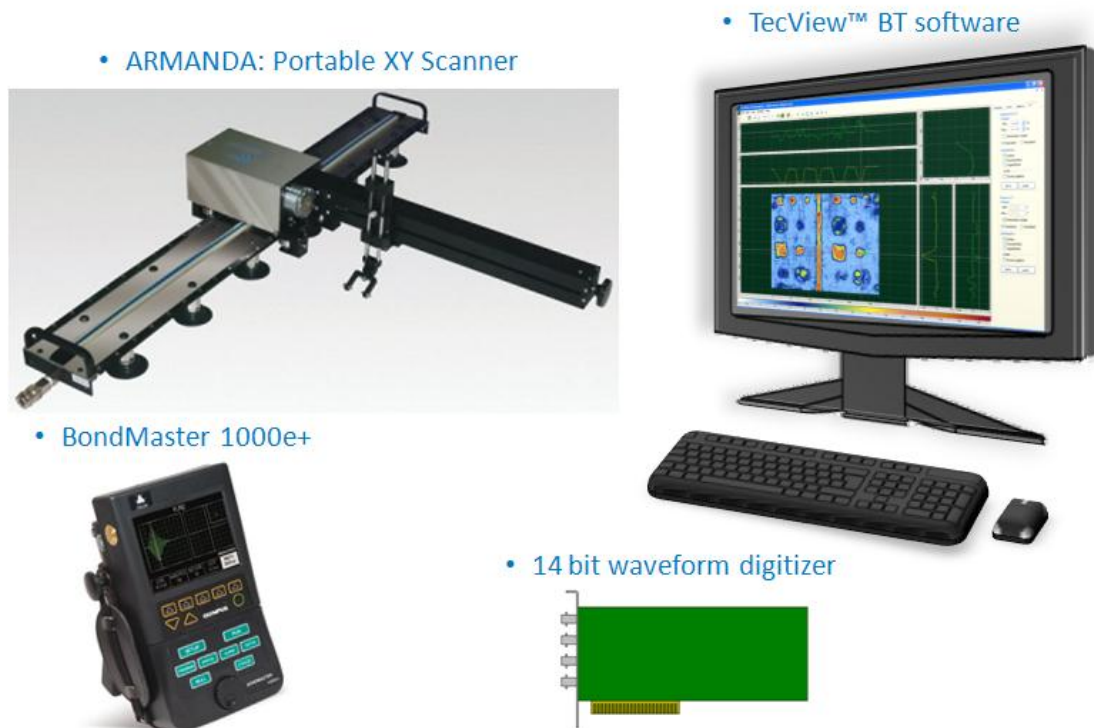
Fig. 6. Experimental setup: ARMANDA scanner, TecView™ BT software, BondMaster 1000e+ and a 14-bit digitizer.
