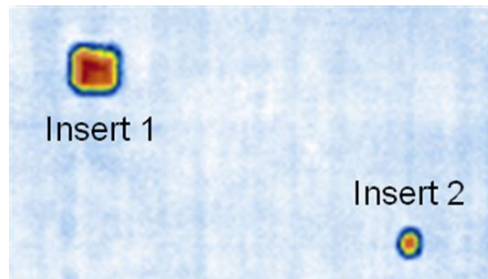
Fig. 7. C-Scan obtained using a conventional 10MHz transducer in pulse-echo mode: approximate area corresponding to the section covered by the resonance probe.
